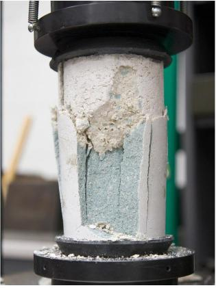
saw how strong our first baseline mix was. It had a compressive strength of ~1000 psi. As a team, we noted very strange irregularities within the concrete as revealed by the compression test. The modified Escape mix had a strange two toned color to it, and we decided to try out new mixes for the canoe. Furthermore, more underclassmen attended this event, and gained knowledge of concrete testing.
